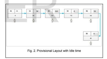
In this "L" shaped layout where total idle time is (21+7.8+10.5+ 6+7.5+9) or 61.8 second. To reduce the total idle time for profitable growth a layout has been proposed for where time is optimized and worker numbers are reduced. In the existing layout, no smoothness was present in operation processes.
